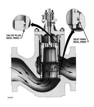
Figure 3. Whisper Trim<sup>®</sup> III Cage in NPS 12 x 8 Design EWNT-2 Valve with Seat Ring Threaded Into the Cage
