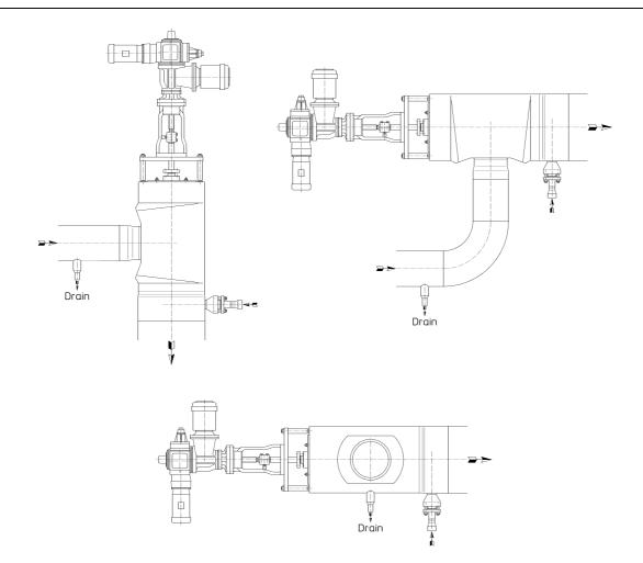
It is also important to protect the downstream system. The connection has to be at lowest point after the valve. It has to be avoided that the valve is at the low point because water can accumulate and cause serious damage. A minimum slope of 1% is recommended (see Piping).
