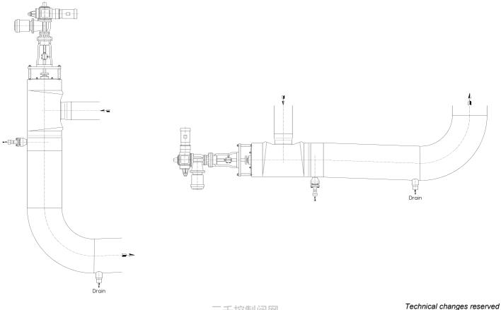
The required straight piping length (see piping downstream) has to be considered but also a malfunction of the temperature sensor (see temperature sensor) has to be avoided.
