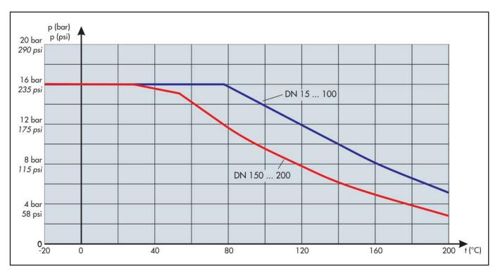
Fig. 6: Pressure-temperature diagram, PN 16
