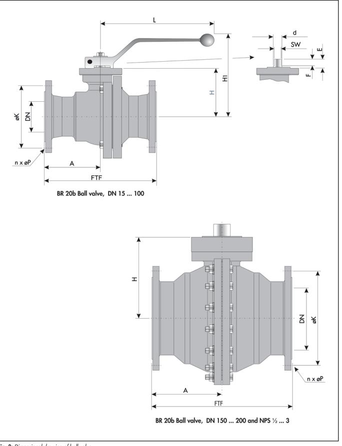
Fig. 8: Dimensional drawing of ball valve
